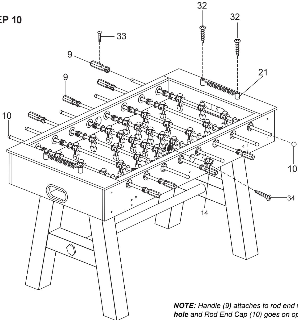
**NOTE:** Handle (9) attaches to rod end with **hole** and Rod End Cap (10) goes on opposite end. Each team should **face the opposite goal** and all be the **same color**. See diagram above for rod and player positions.
