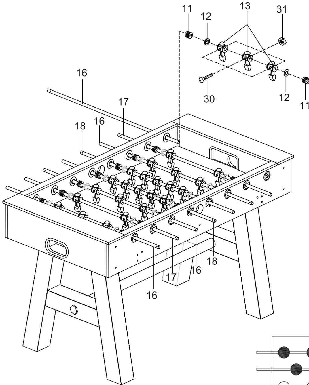
*Insert rod end part way through one side panel, then place rest of parts needed on each rod, in order shown, before inserting through other side panel.*
