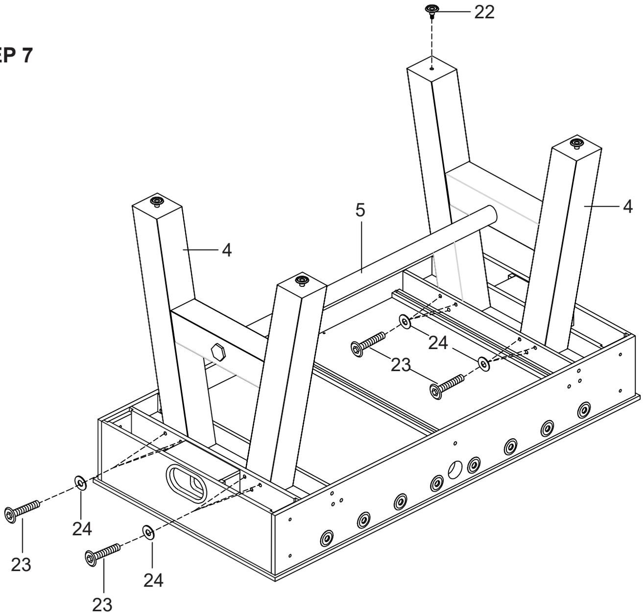
**NOTE:** Two adults are required to turn table upright. Turn over using main table body only, NOT legs, and place on all four feet on ground at same time.
