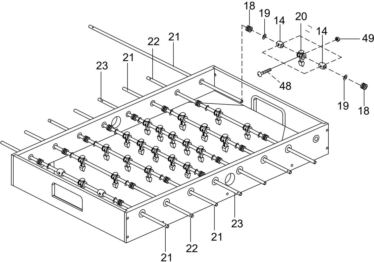
*Insert rod end part way through one side panel, then place rest of parts needed on each rod, in order shown, before inserting through other side panel.*
