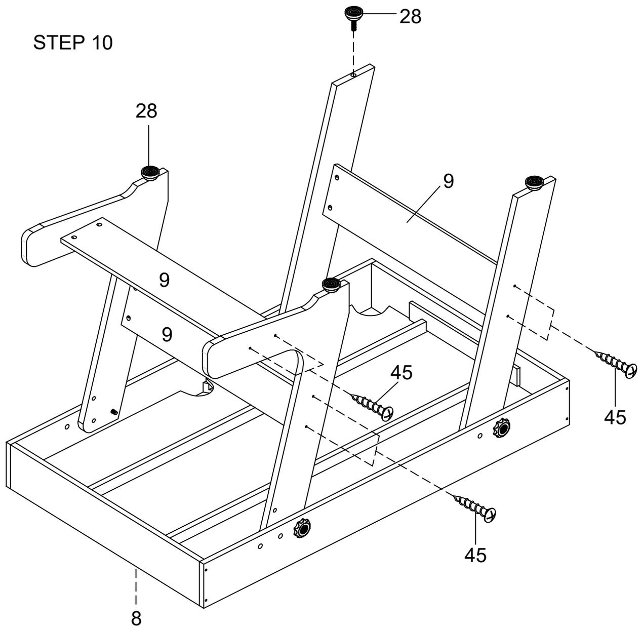
**NOTE:** Two adults are required to turn table upright. Turn over using main table body only, NOT legs, and place on all four feet on ground at same time.
